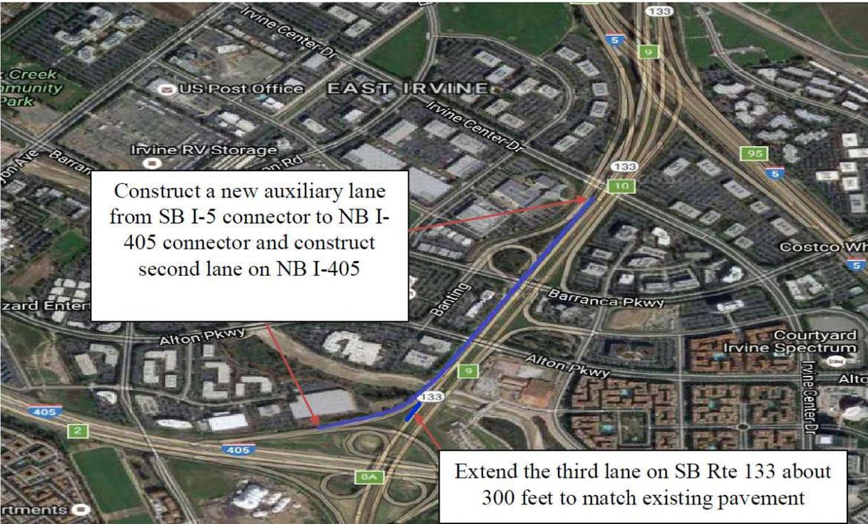
**Build Alternative** New Auxiliary lane from SB Rte 133/SB I-5 connector to SB Rte 133/ NB I-405 connector and construct second lane on SB Rte 133/ NB I-405 Connector
