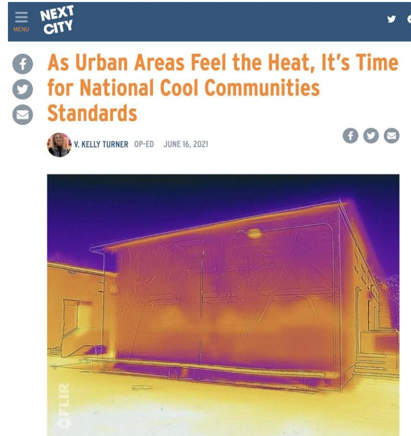
Thermal color image of Kristy Sandoval's "Beat the Heat" mural at Fernangeles Elementary School in Pacoima, in Los Angeles. The mural uses solar reflective paint to lower the temperature of the wall from over 100 degrees F to as low as 86 degrees F. Purple indicates cooler temperatures whereas red/yellow signals hotter temperatures, such as the asphalt, which registered 136 degrees F. (Photo by Ariane Middel, ASU)
